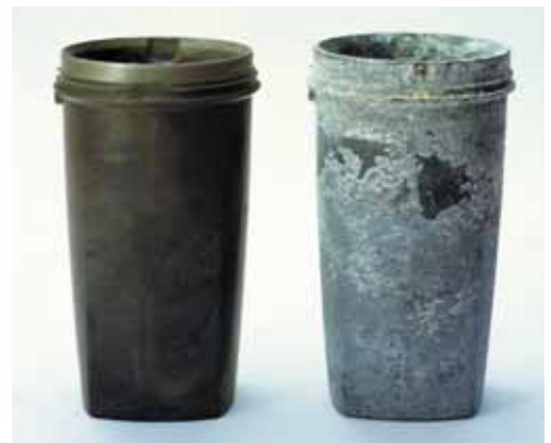
Alocrom Treated Untreated Aluminum
