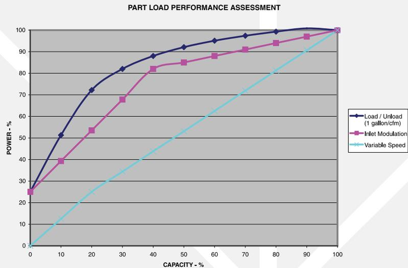
Variable Speed Drive is the superior alternative to other compressor control systems. The chart above represents the nominal control systems for generic comparative purposes. A detailed and accurate comparison of specific compressor models is available from your Sullair representative or authorized distributor.
